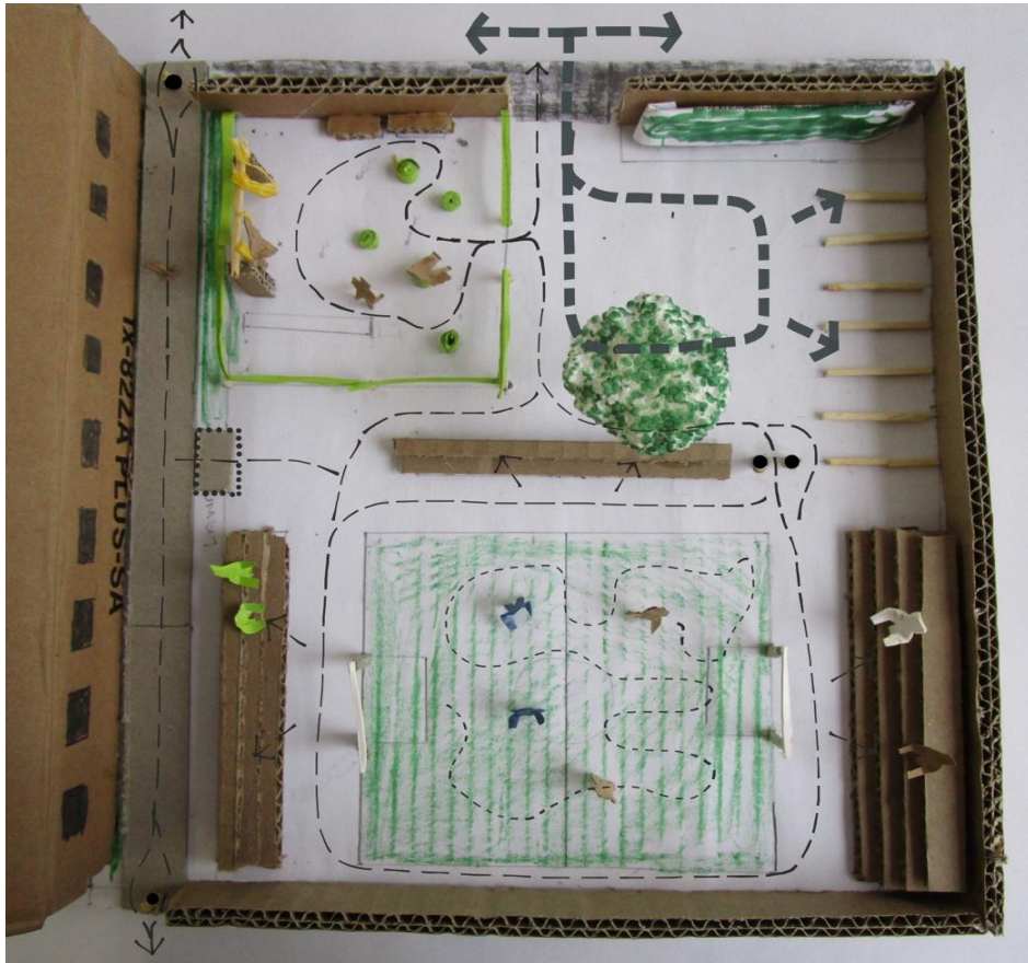
Figure 4: Analysis of movement routes in Sonwabo’s Model 4 (Pedestrian routes are shown by thin dashed lines and vehicular movement routes are shown by thick dashed lines)
