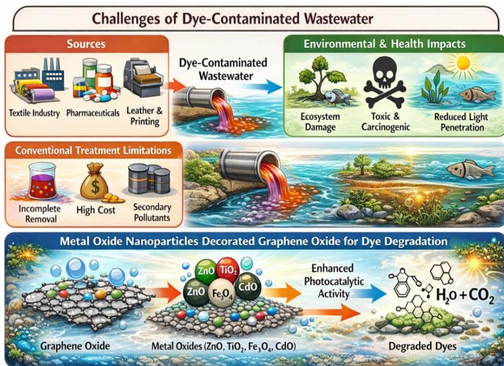
Figure 1: Schematic representation of environmental impacts of dye-contaminated wastewater and the mechanism of photocatalytic degradation by metal oxide-decorated graphene oxide nanocomposites
