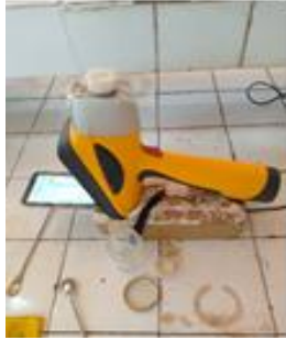
Figure 3: Portable X-ray fluorescence spectrometer
