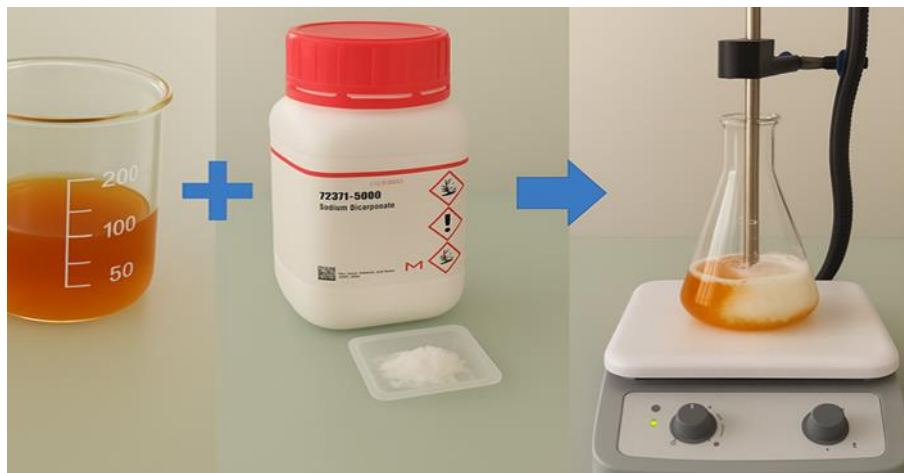
Figure 2: Preparation of the solution and reduction to ZnONPs
