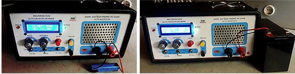
Figure 8: Battery test set-ups: 3.7 V/6 800 mAh Li-ion battery (left) and 12 V/10 Ah lead-acid battery (right)
